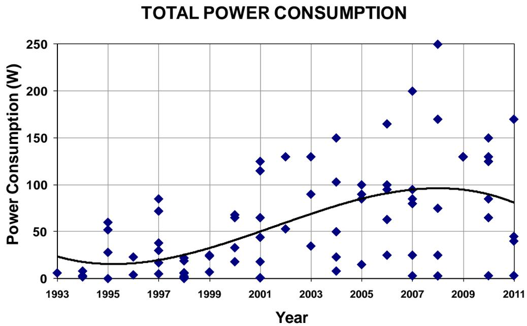
Figure 2: Total microprocessor power consumption vs Year
