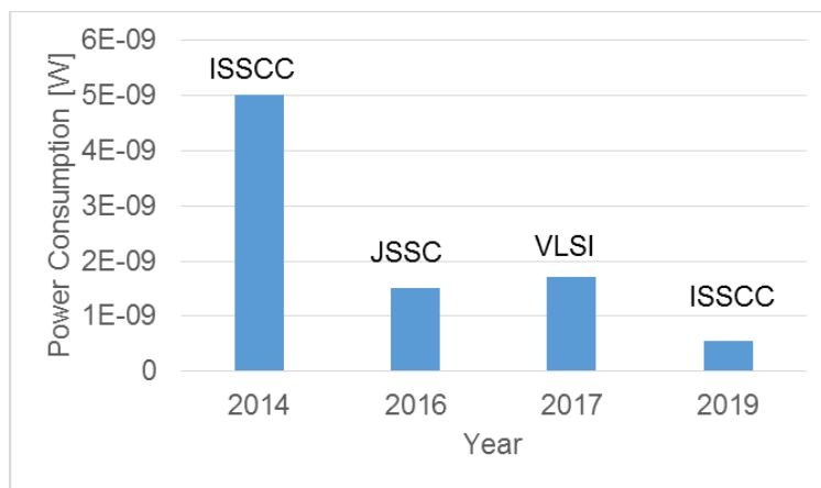
Figure 2 – Trends in Recent Low Power Fast Startup Crystal Oscillators versus Time
